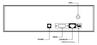
**Power -** 2.5mm dia jack mates with power cord on Ultralink supplied wall mounted power supply.
