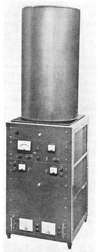
Fig. 6. Photograph of a hydrogen maser frequency standard [20]
