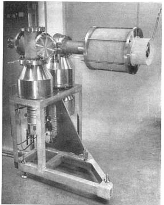
Fig. 4. Photograph of hydrogen maser. The apparatus is about four feet tall. The magnetic shields are removed
