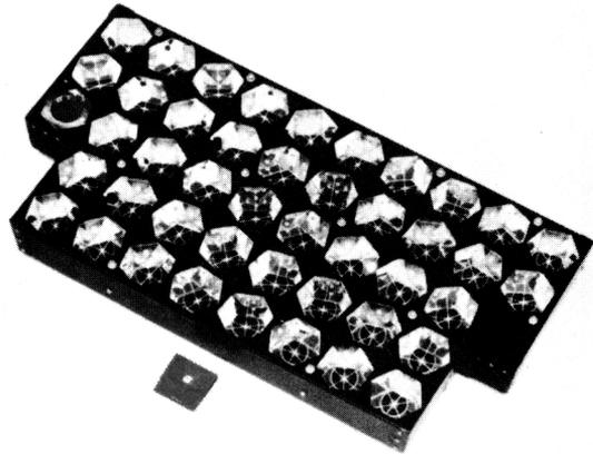
Fig. 35 - NTS-2 laser retroreflector
