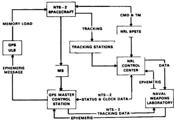
Fig. 7 - NTS-2 command and telemetry links
