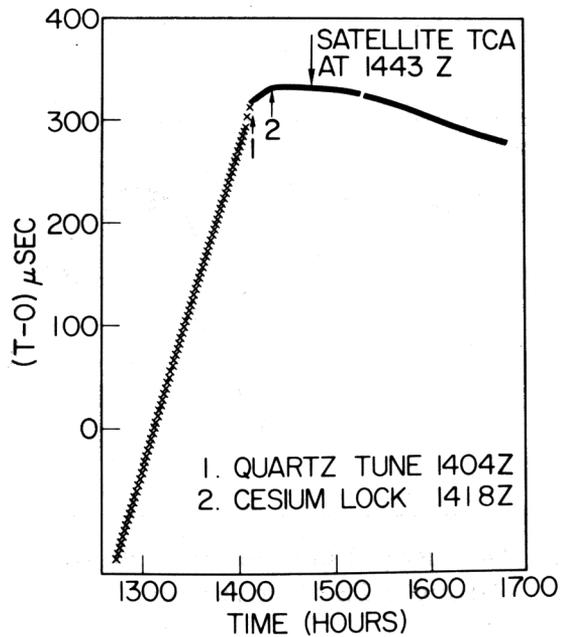
Fig. 19 - Cesium frequency standard lock up, 1977 day 190, 1418 UTC
