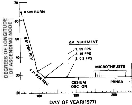
Fig. 9 - NTS-2 drift orbit adjustments
