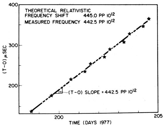
Fig. 20 - Cesium frequency via (T-O) slope
