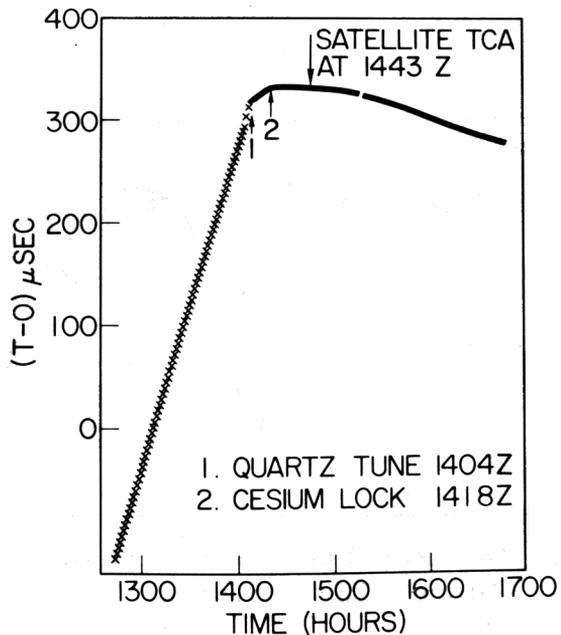
Fig. 19 - Cesium frequency standard lock up, 1977 day 190, 1418 UTC
