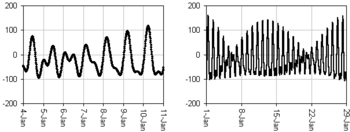
The plots clearly reveal multiple cycles superimposed. To better understand this, the first plot below is the solar-only component of the 1-week plot above; the second plot below is the lunar-only component.
