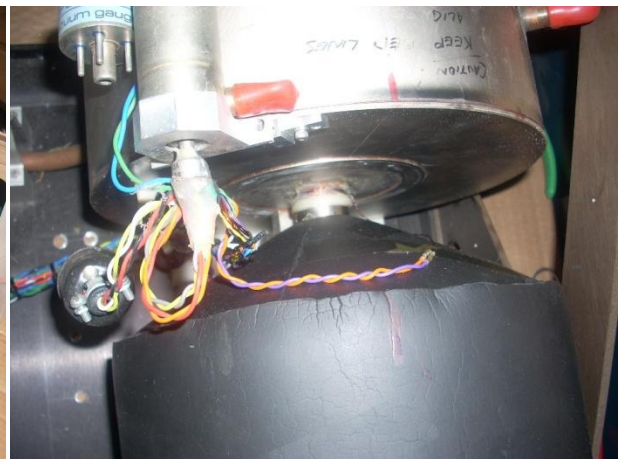
Solid state pressure sensor on canister
