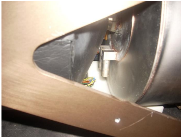
One set of the liquid cooling ports
