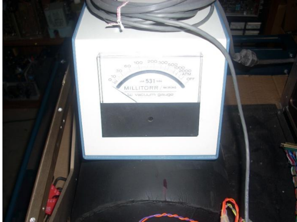
Vacuum reading using 531 TC gauge tube
