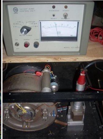
Vacuum reading using ion pump current
