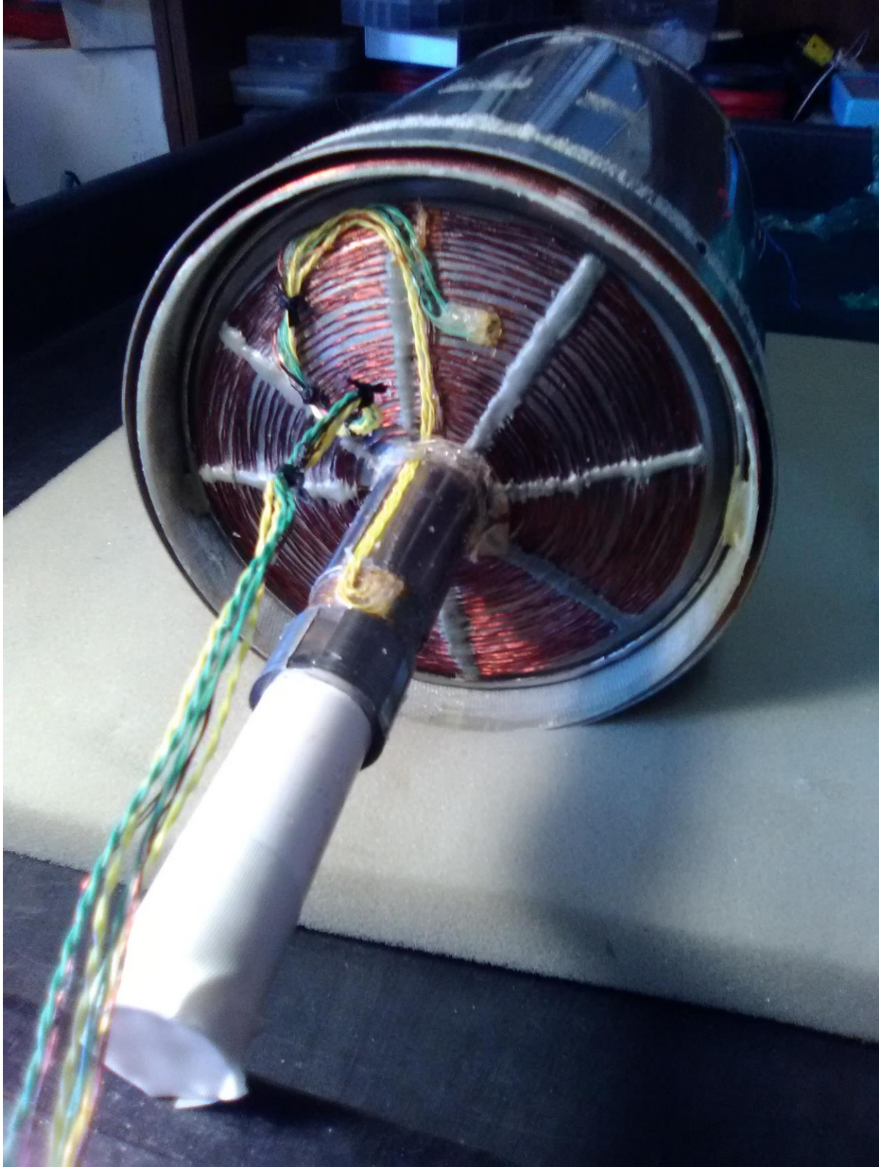
VACUUM ENVELOPE END HEATER. SMA CABLES SHIELDED PRIOR TO CUT
