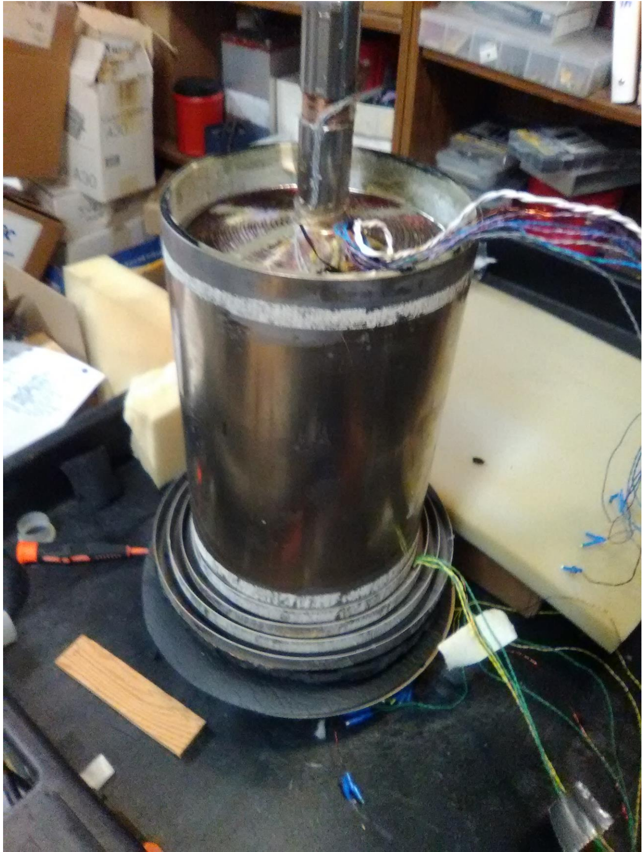
VACUUM ENVELOPE END HEATER AND LAST SHIELD
