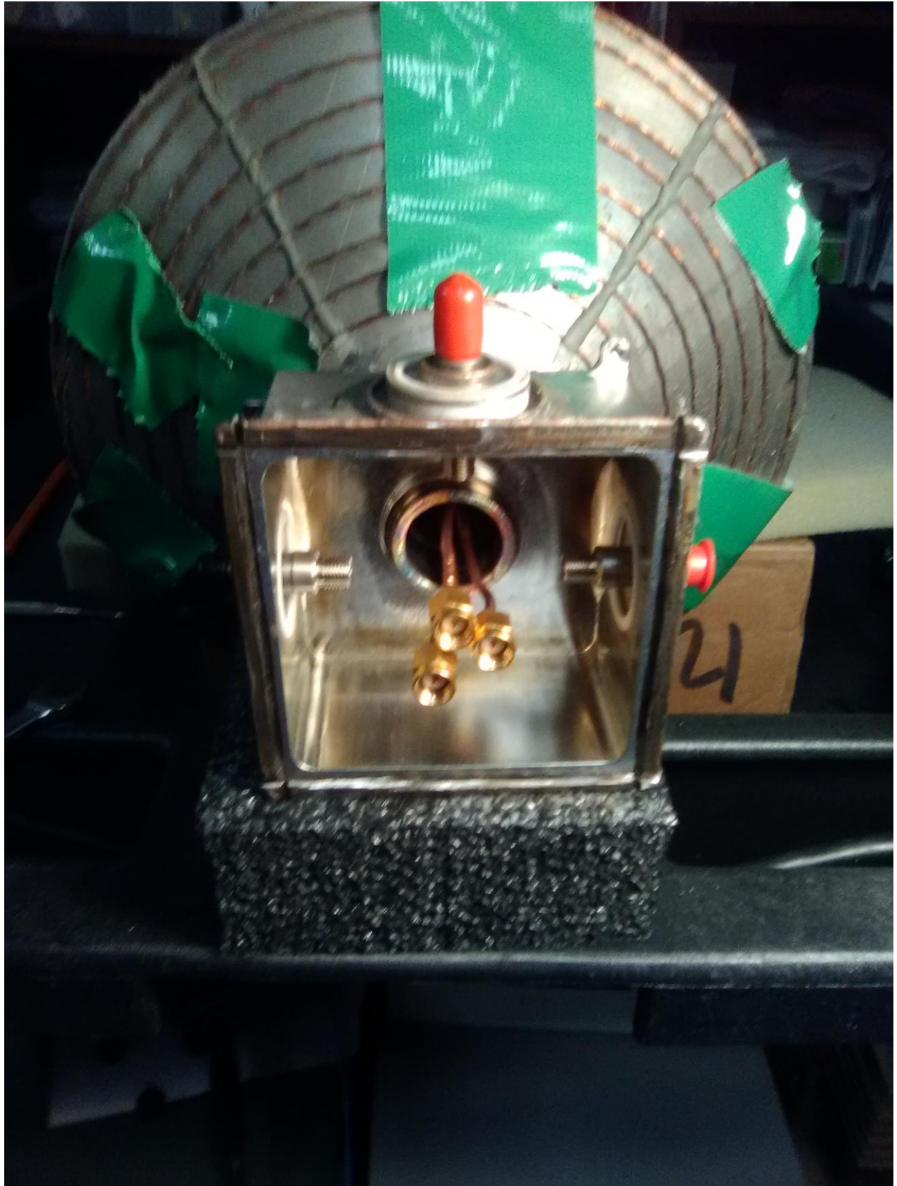
RF BOX SMA DISCONNECTED
