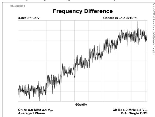
It is not known at this point if the short- and long-term cavity auto-tuning charts are nominal for this model of maser. Or are they unique to the one in my lab, or a side effect of less than perfect environmental control, or some sort of interaction between two cavity-tuning masers?
