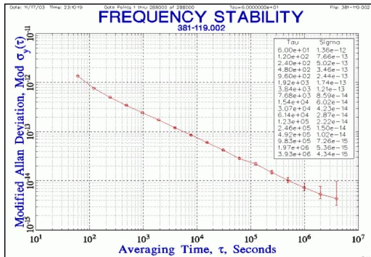
The following plot of two active hydrogen masers (Sigma Tau vs. KVARZ) shows stability below  $2 \times 10^{-15}$  at 10,000 seconds.
